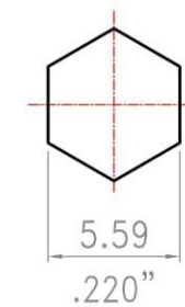
Recommended Crimped Dimensions for Ferrule
