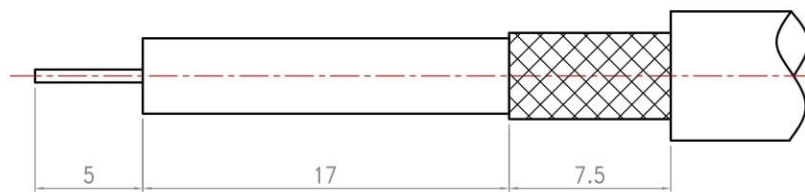
Recommended Cable Stripping Dimensions
