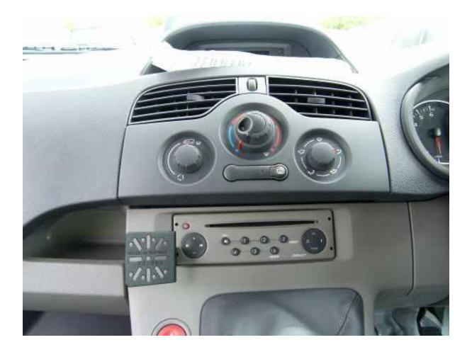
Step 1: Unclip the fascia panel from around the gear shift and radio.
