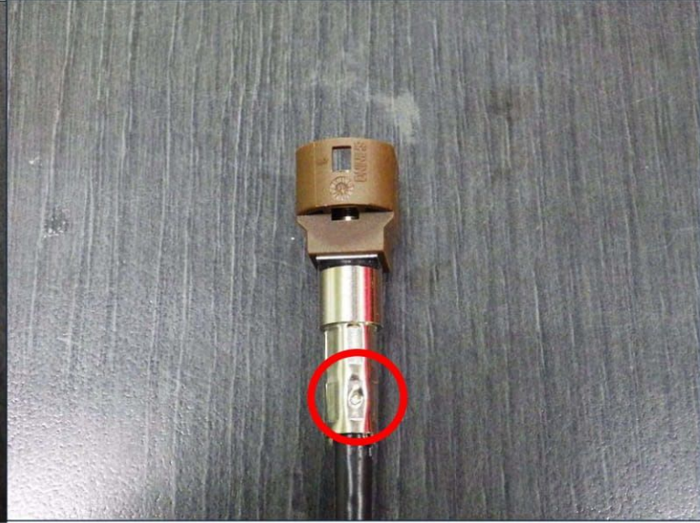
Crimping ferrule done for HSD Male connector.
